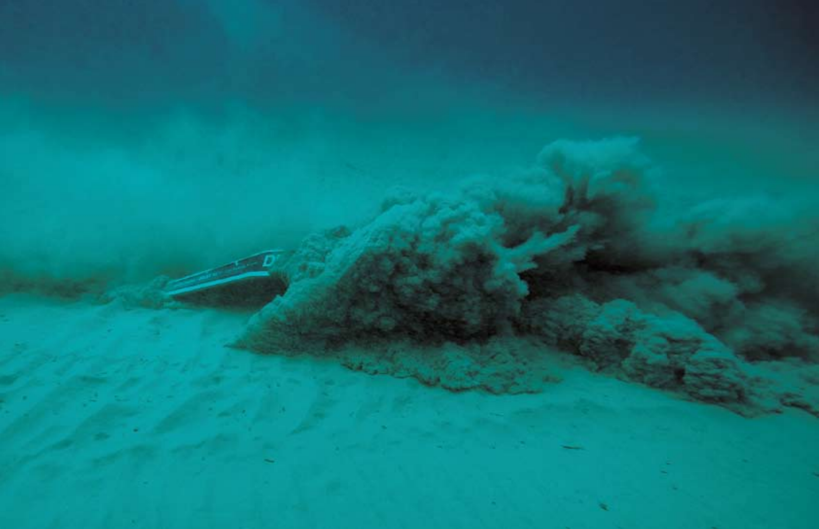
Lewmar Delta: this new-generation anchor is fitted as standard by many boatbuilders, but tends to plough the seabed without digging in deeply
