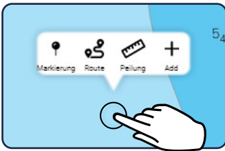
Fig.11: Long press and hold opens quick menu to create a marker, route, bearing or POI
