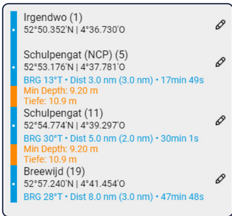
Fig.13: Display of route segments with distances from start to the particular WP and each segment distances (in brackets).
