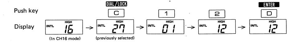
The channel numbers other than above are invalid and cannot be accepted. In this case, by pushing the ENTER key, the entered number is canceled and the display will retain the previous channel number.
