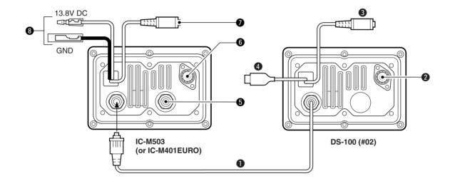
**NOTE:** Binding the GPS cable, GPS connector, clone receptacle, antenna connector with water-resistant tape, increases the waterproofing of the controller.
