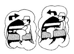
For smooth steering, adjust the steering friction bolt so that a slight drag is felt when turning.
