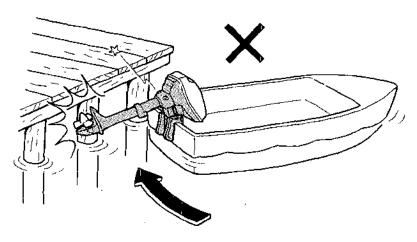
CAUTION: To avoid damaging the motor, never use it as a handle for lifting or moving the boat.
