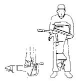
Transport and store the motor either vertically or horizontally, as shown here, with the steering handle raised.
