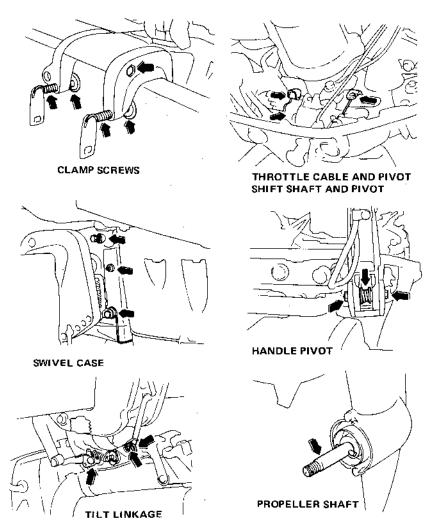
NOTE: Apply anti-corrosion oil to pivot surfaces where grease cannot penetrate.
